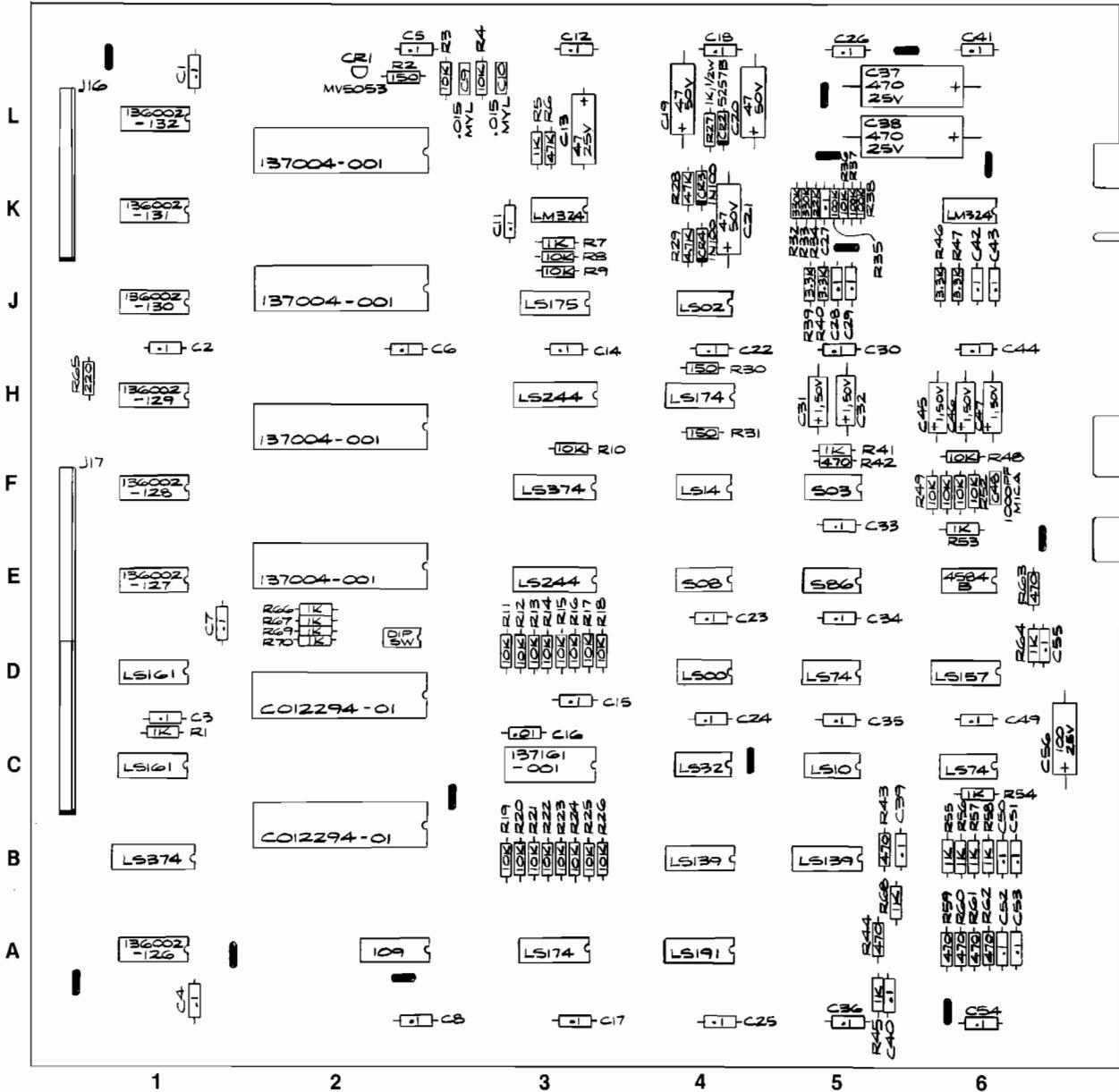
Figure 22 Tempest™ Auxiliary PCB Assembly
