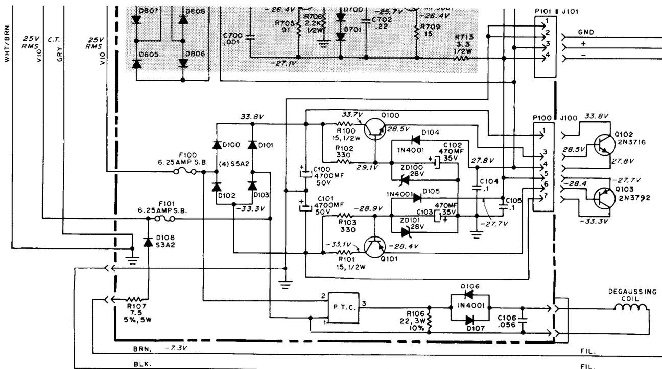
Figure 7 Schematic Diagram of Low-Voltage Power Supply
