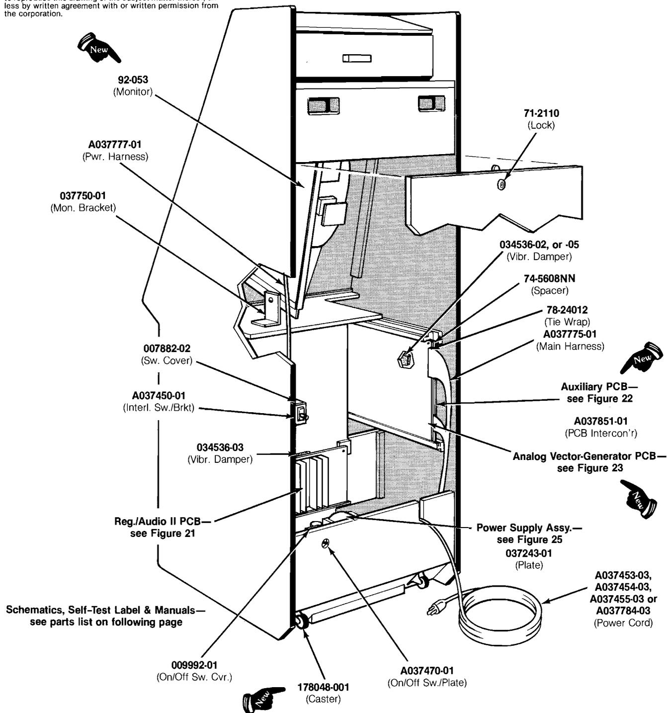
**Figure 18 Cabinet-Mounted Assemblies**
