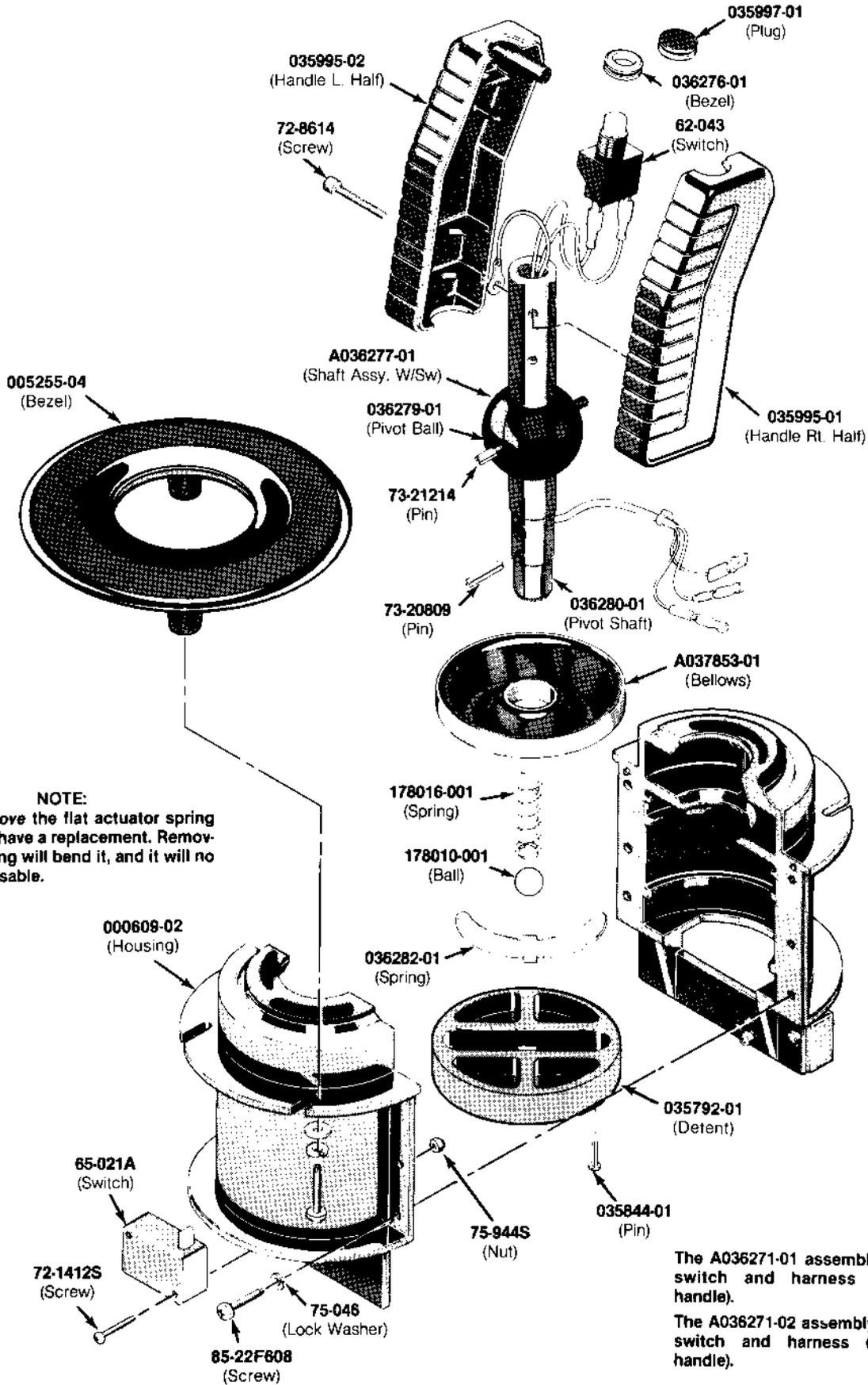
The A036271-01 assembly has NO fire switch and harness (left control handle).
