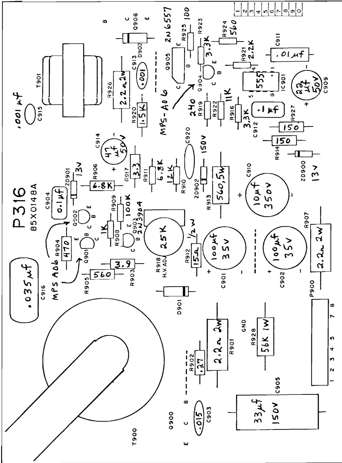
Figure 15 High-Voltage PCB Assembly
