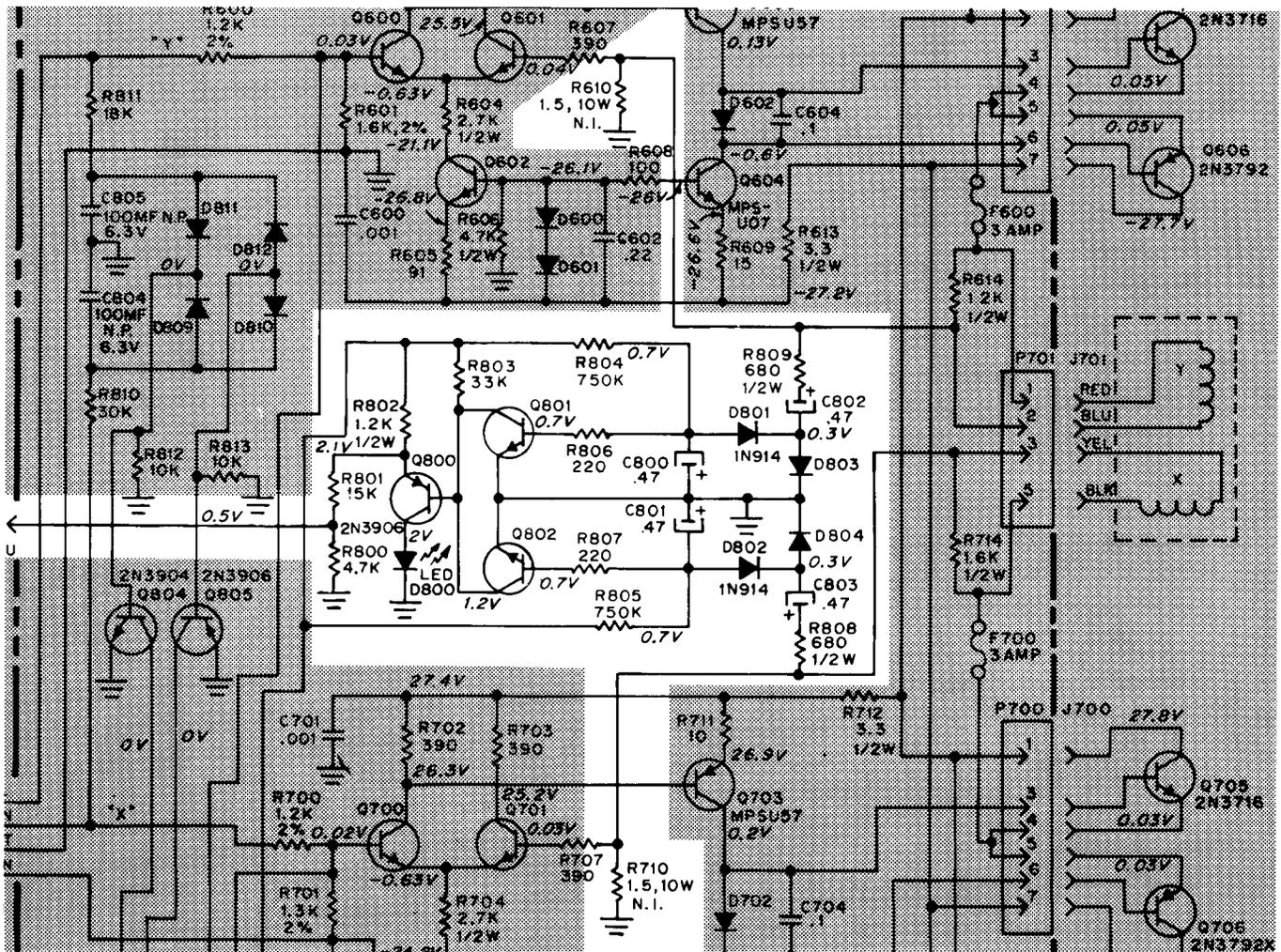
Figure 11 Schematic Diagram of Spot Killer Circuitry
