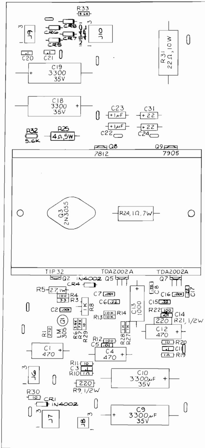
**Figure 21 Regulator/Audio II PCB Assembly**
