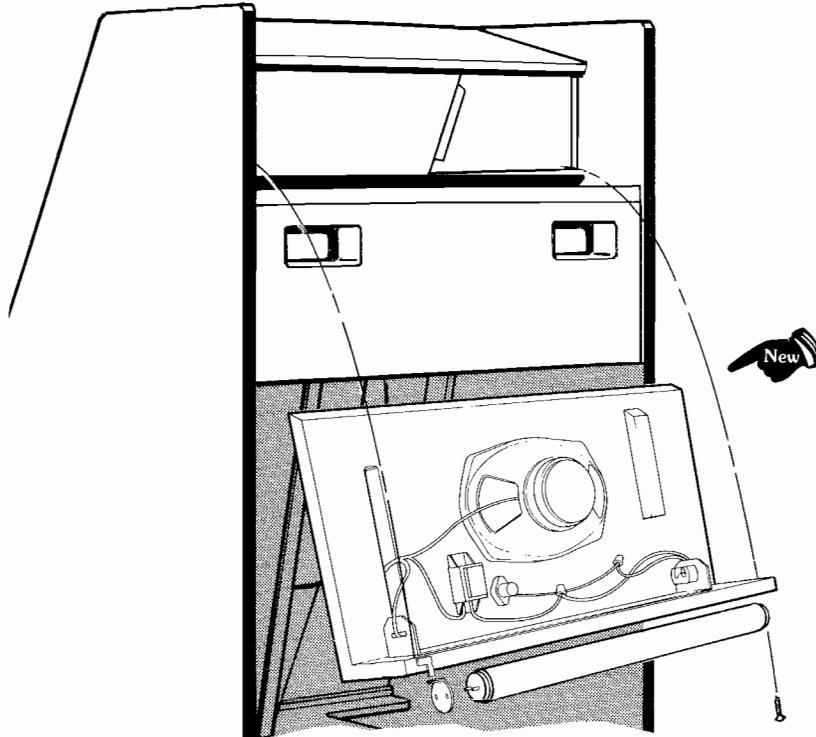
Figure 14 Fluorescent Tube and Speaker Replacement
