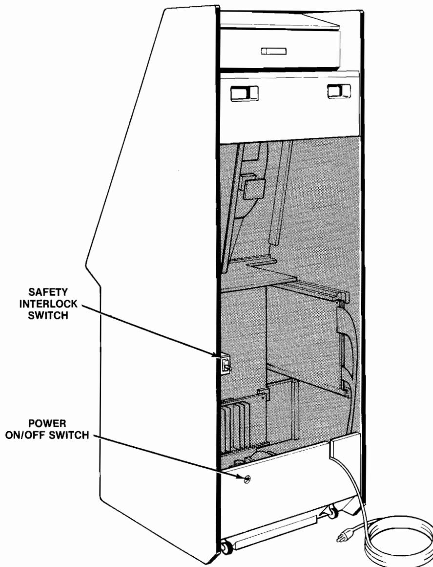
**Figure 4 Interlock and Power On/Off Switches**
