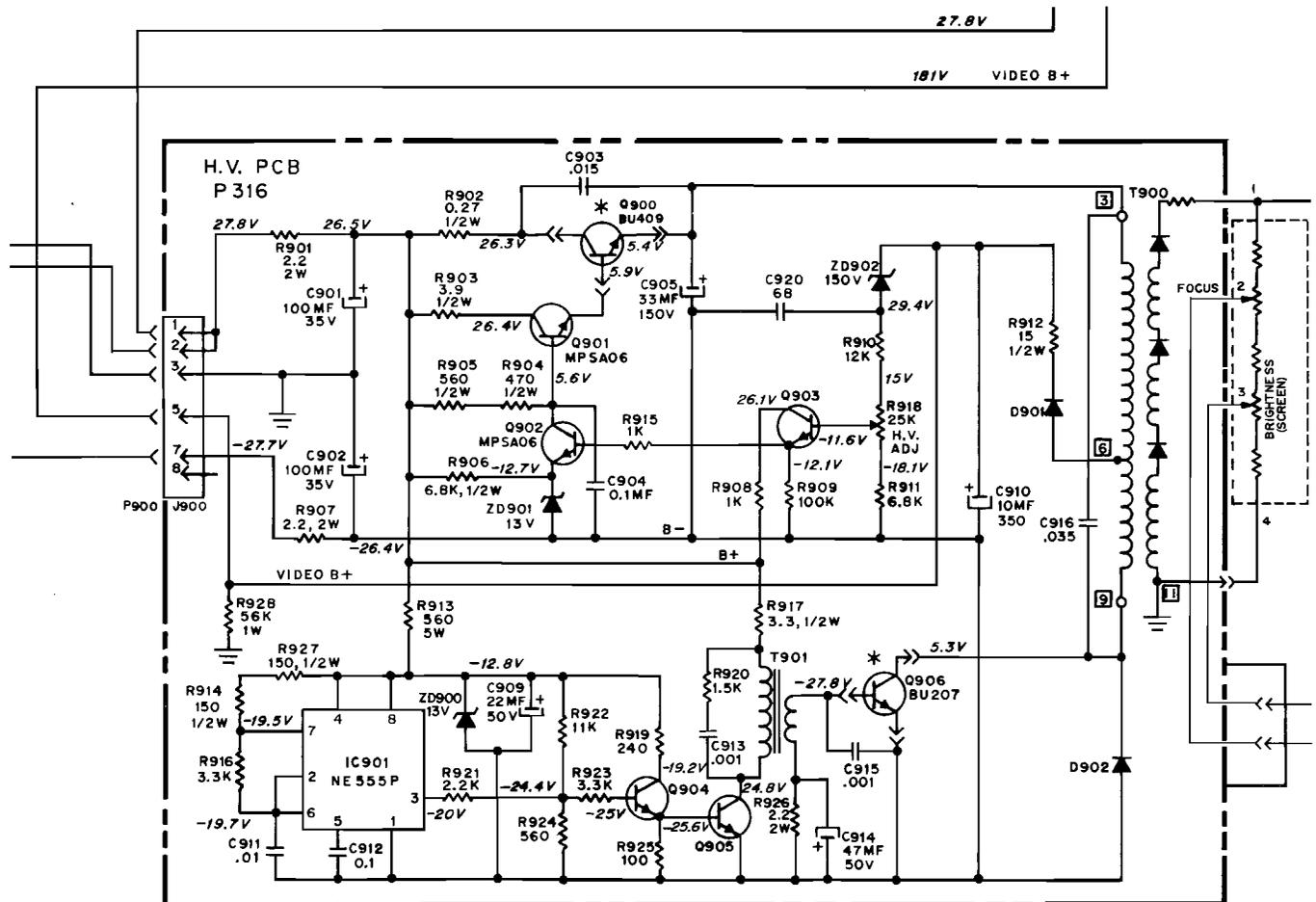
Figure 10 Schematic Diagram of High-Voltage Power Supply
