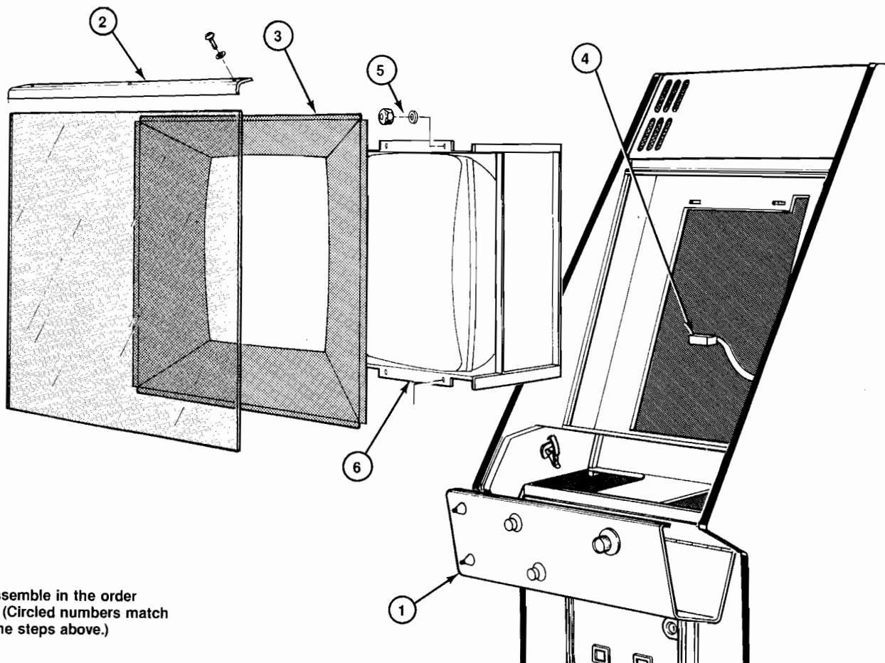
Figure 13 Monitor Removal
