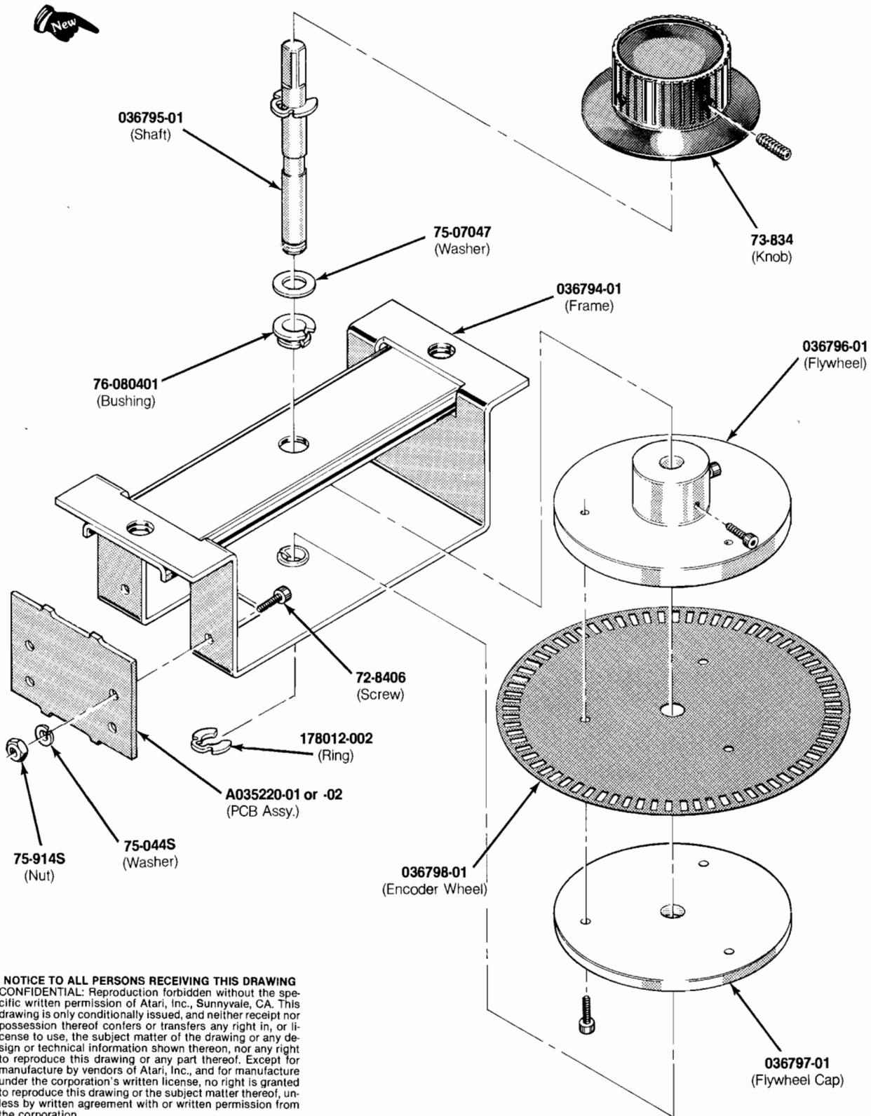
**Figure 20 Encoder Wheel Assembly
