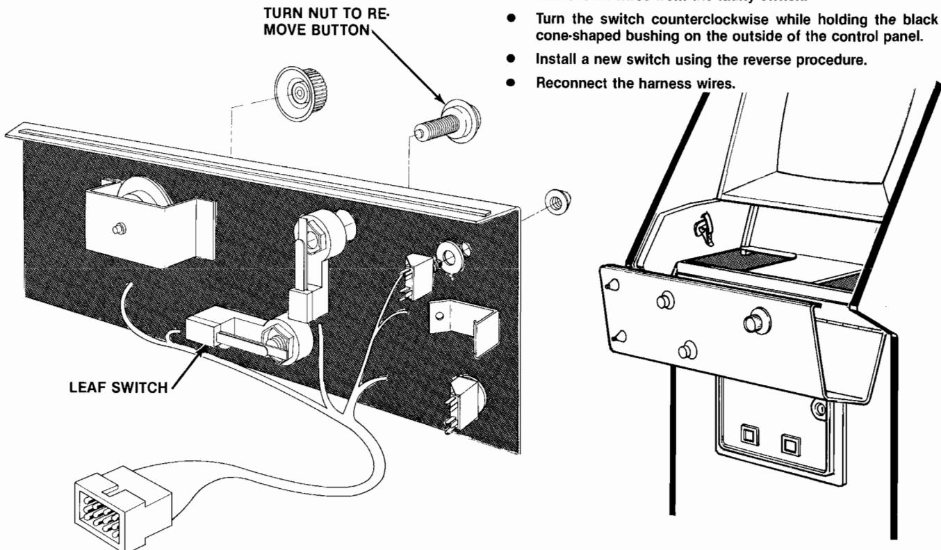
Figure 10 Opening the Control Panel and Replacing Switches
