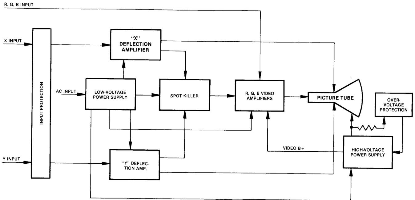
**Figure 6 Display Block Diagram**
