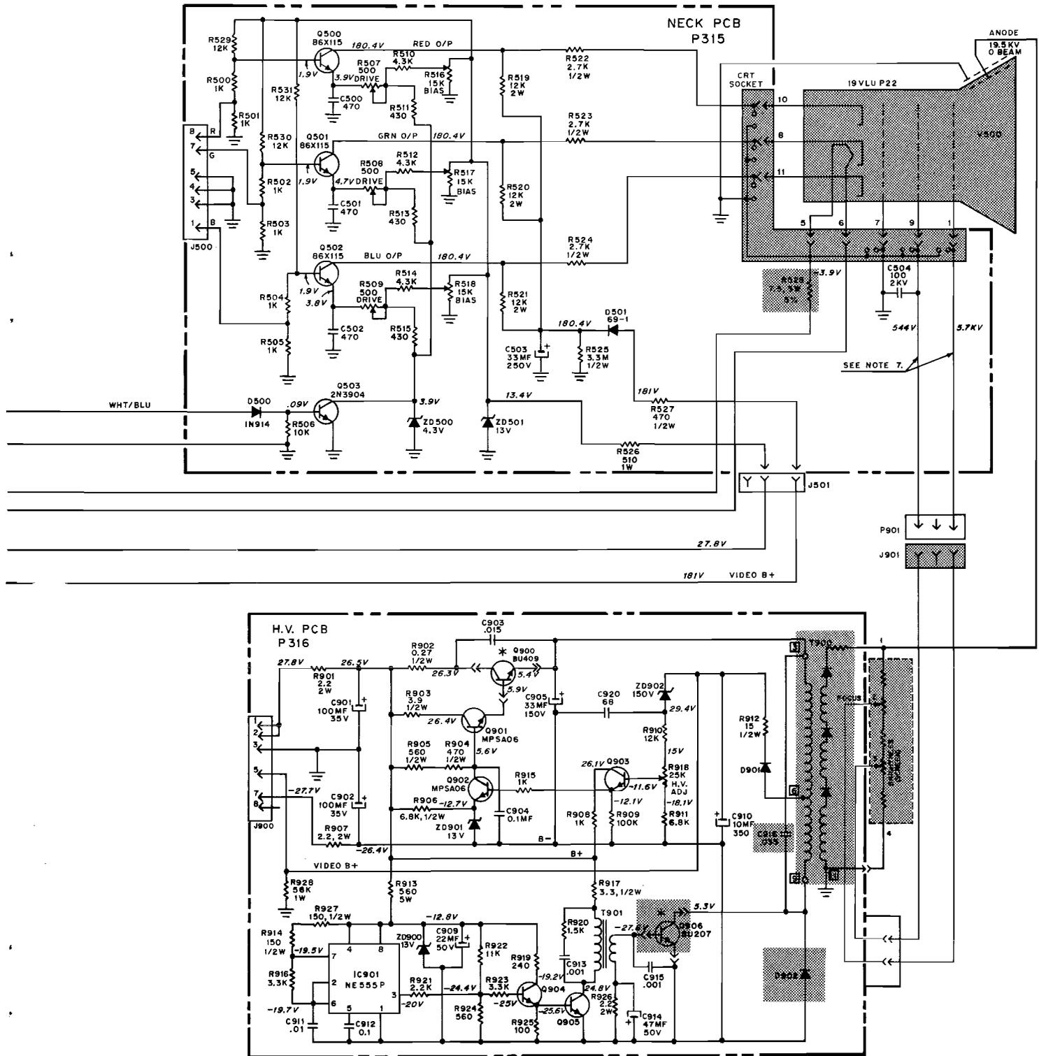
Figure 11 Display Schematic Diagram
