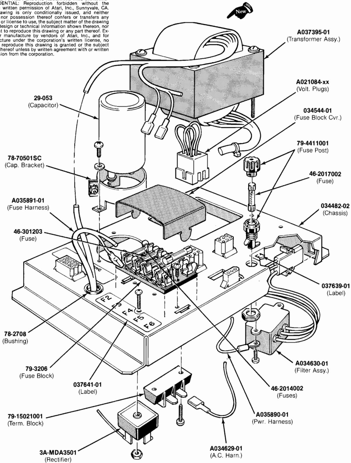
**Figure 25 Color X-Y Power Supply Assembly**
