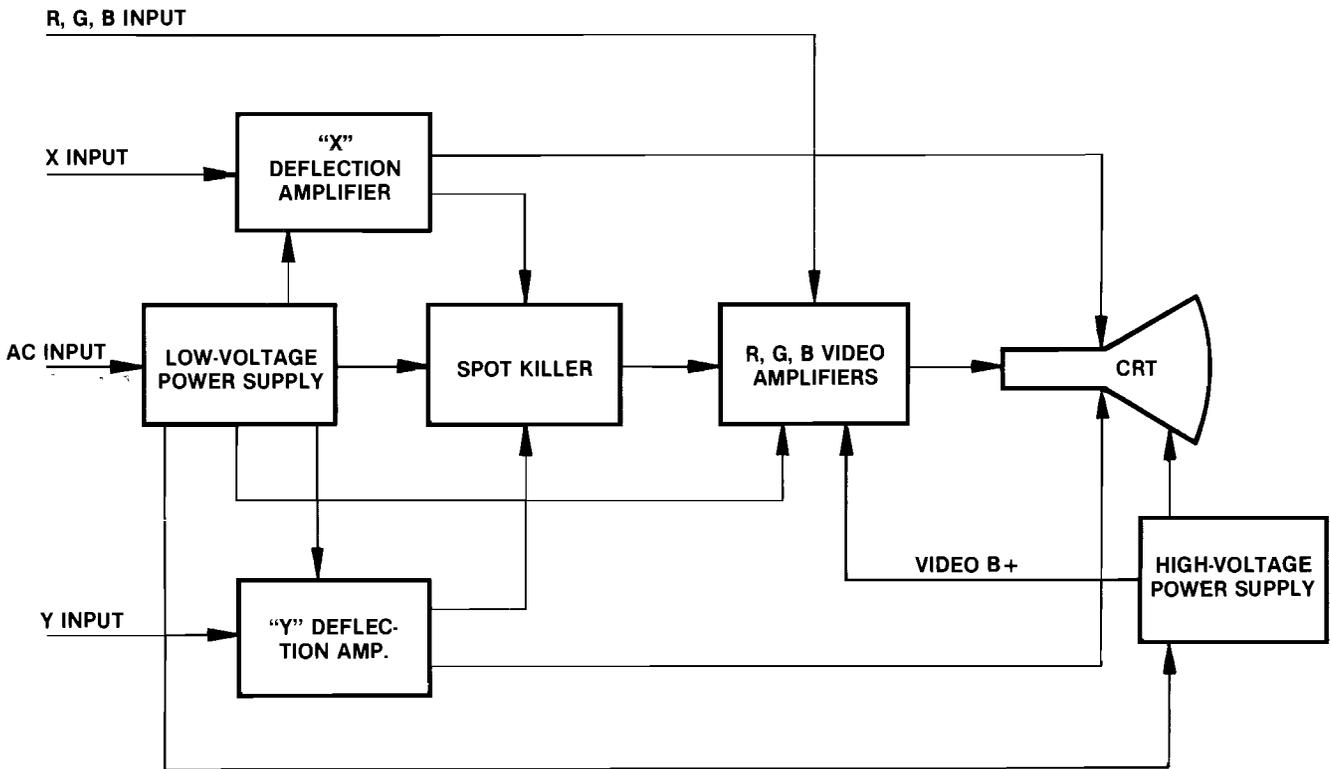
Figure 5 Display Block Diagram
