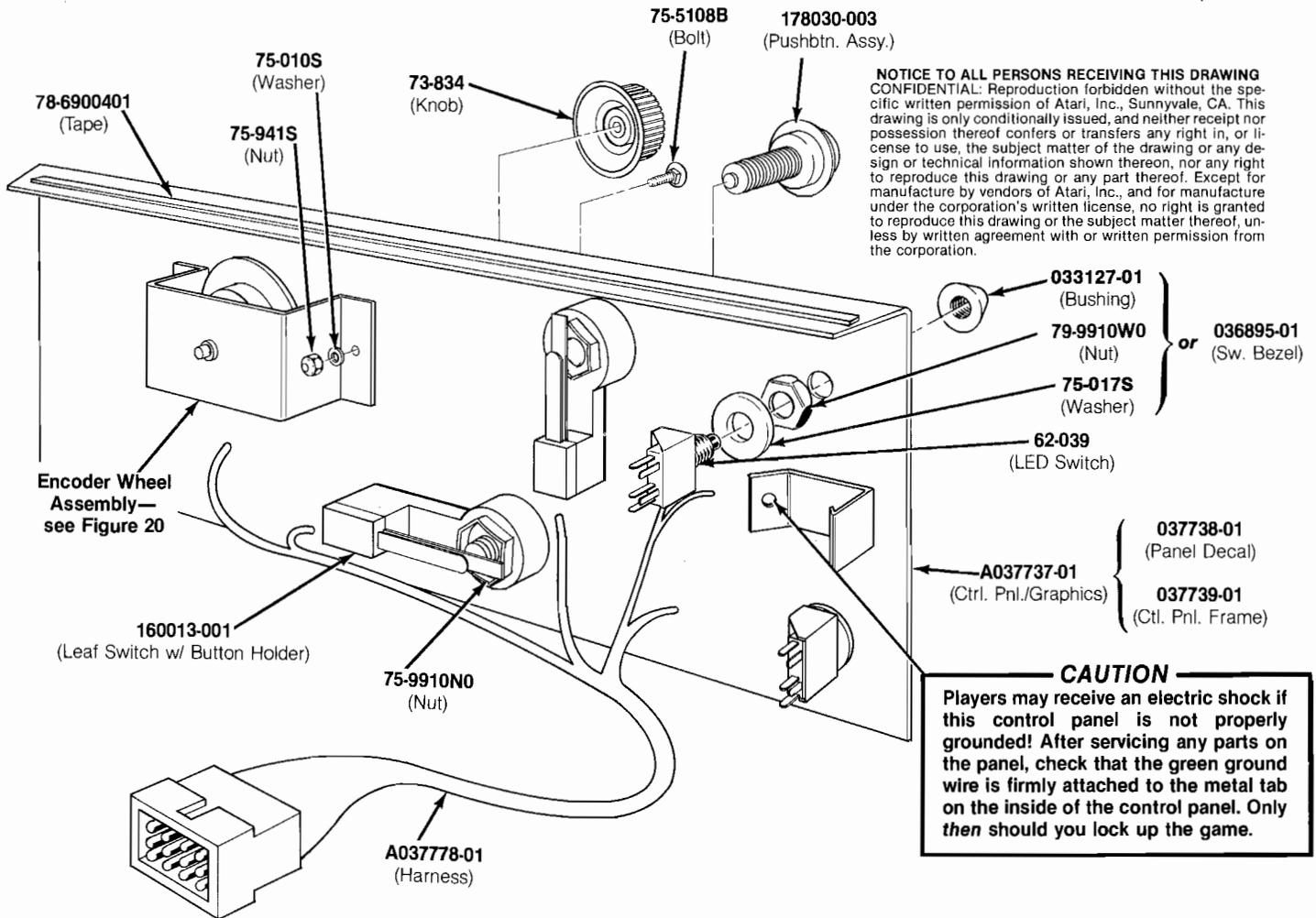
**Figure 19 Control Panel Assembly
