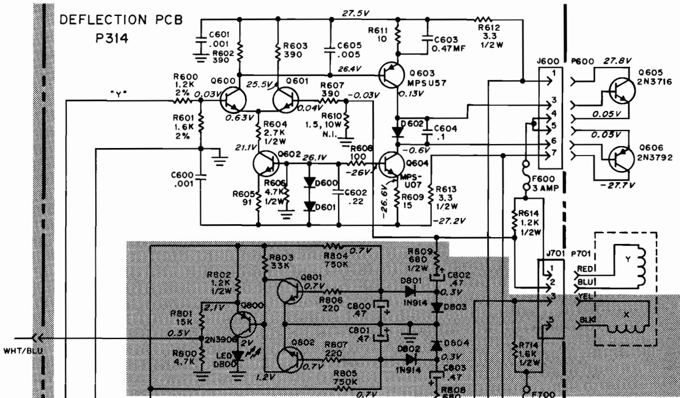
Figure 7 Schematic Diagram of Y Amplifier
