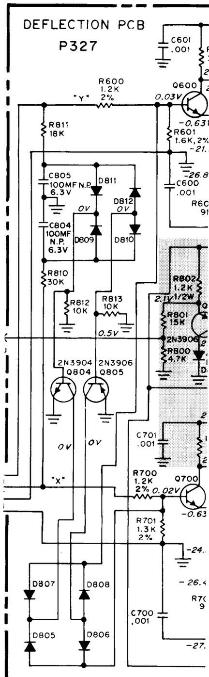
**Figure 8 Schematic Diagram of Input Protection**
