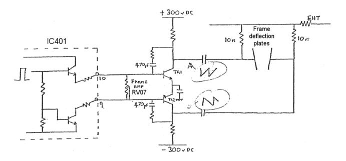
During frame flyback transistors T52 and T50 are turned on. This causes the transistors TR1 and TR2 to turn on and eventually saturate.
