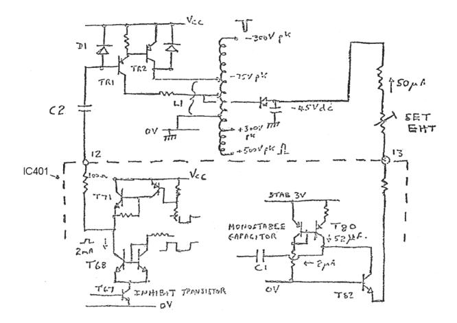
Energy is stored in L1 during part of the line scan period and is then released into the various parts of the circuitry suring line flyback time.
