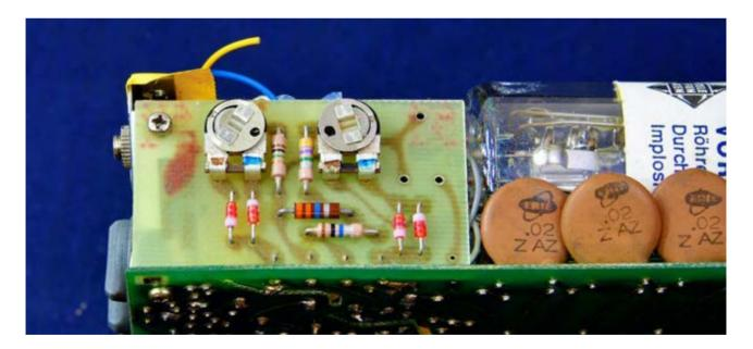
As an aside, note the extremely high value resistors, of up to  $33M\Omega$ . Even higher values are employed on the main board.
